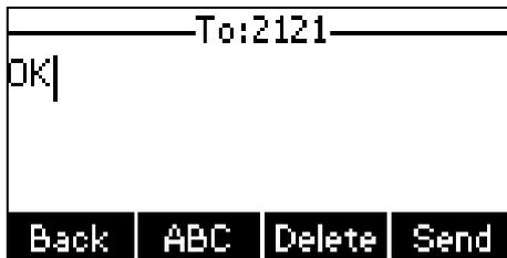
3. Compose the new text message. You can press the **abc** soft key to change the input mode.
