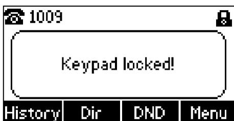
You can configure the interval (in seconds) to automatically lock the keypad instead of long pressing
